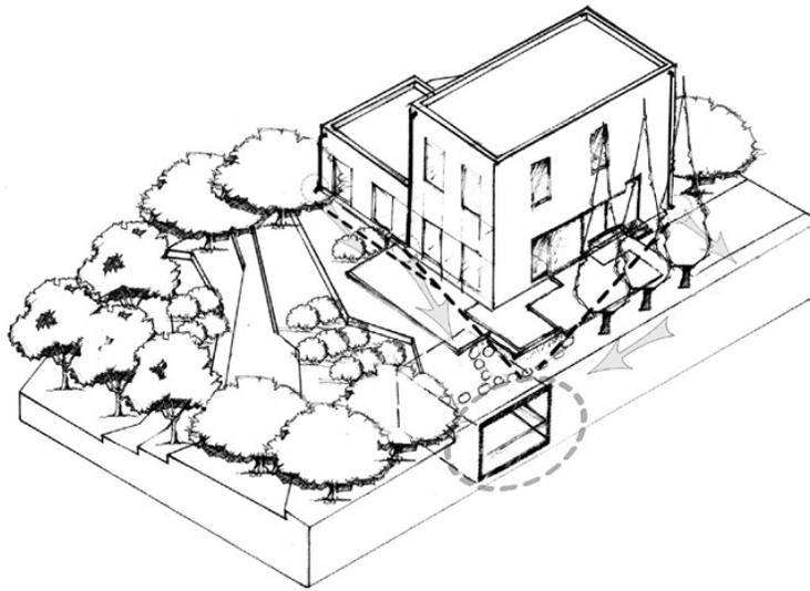
**Fig. 3.8: An active rainwater harvesting system.**
