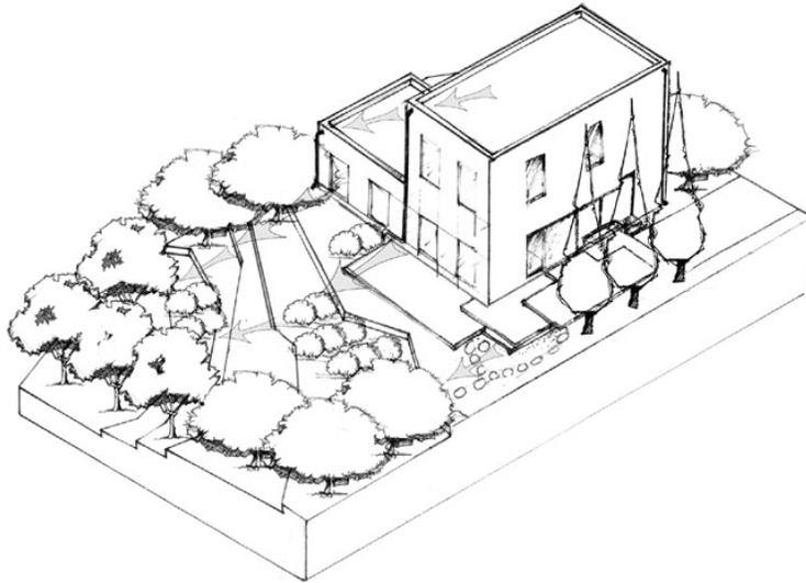
**Fig. 3.5: A site plan showing an analysis of rainfall drainage.**
