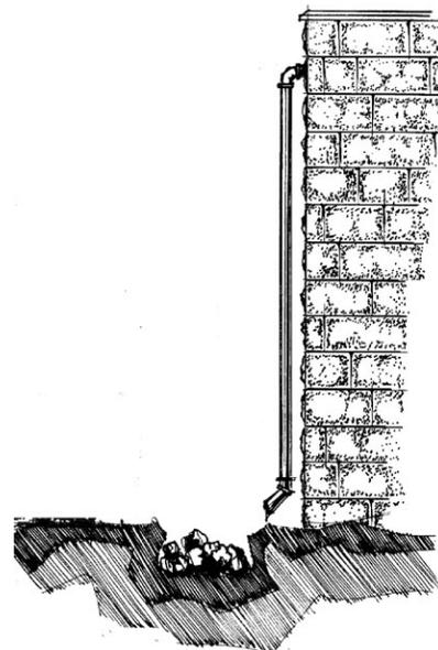
**Fig. 3.6: Rocks may be used to disperse water coming out of a downspout.**
