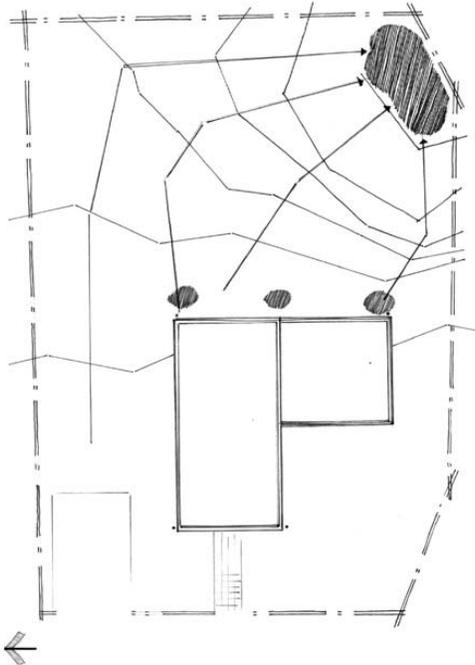
**Fig 3.4: A site plan showing an analysis of rainfall drainage.**
